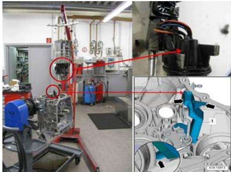
Figure 2. Caution points: drip tray and sensor module connector.
